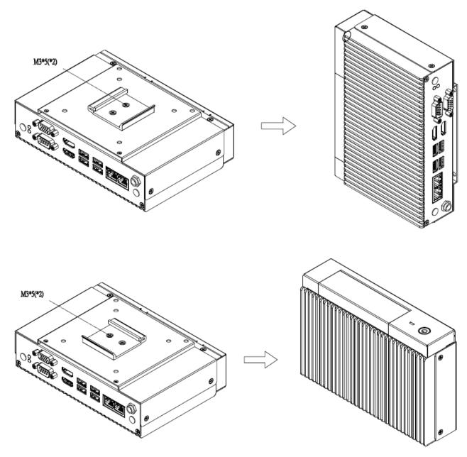
Step1. Position brackets on both sides, matching the holes on the system.
