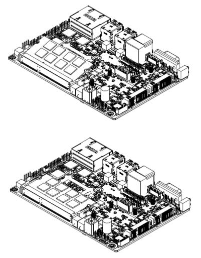
**Step2.** Properly install the memory module and press until properly seated.
