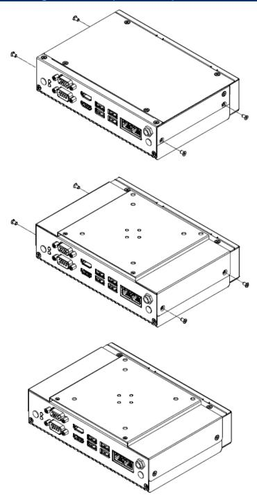
**Step1.** Remove 4 screws from the side.
