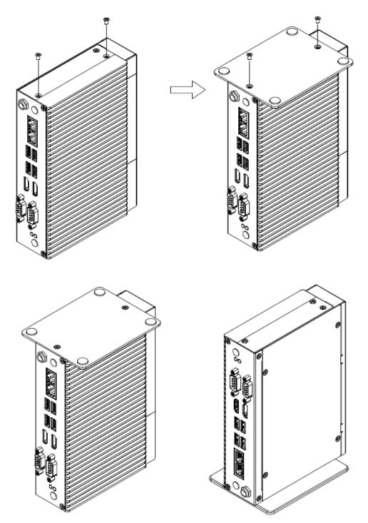
**Step1.** Remove 2 screws from the side.
